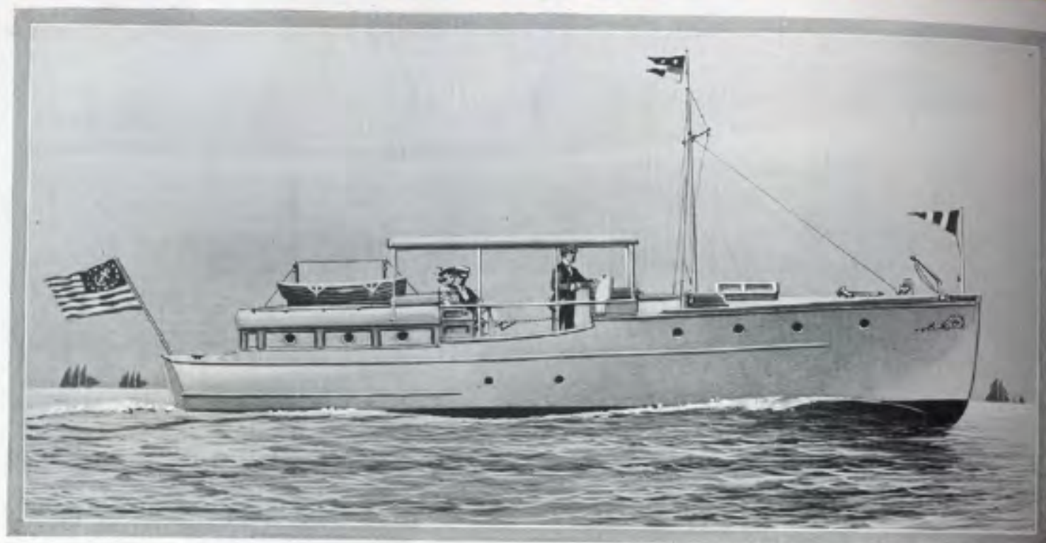
40-foot CRUISETTE, 36-40 Horse Power ELCO Engine. Speed 10 miles
