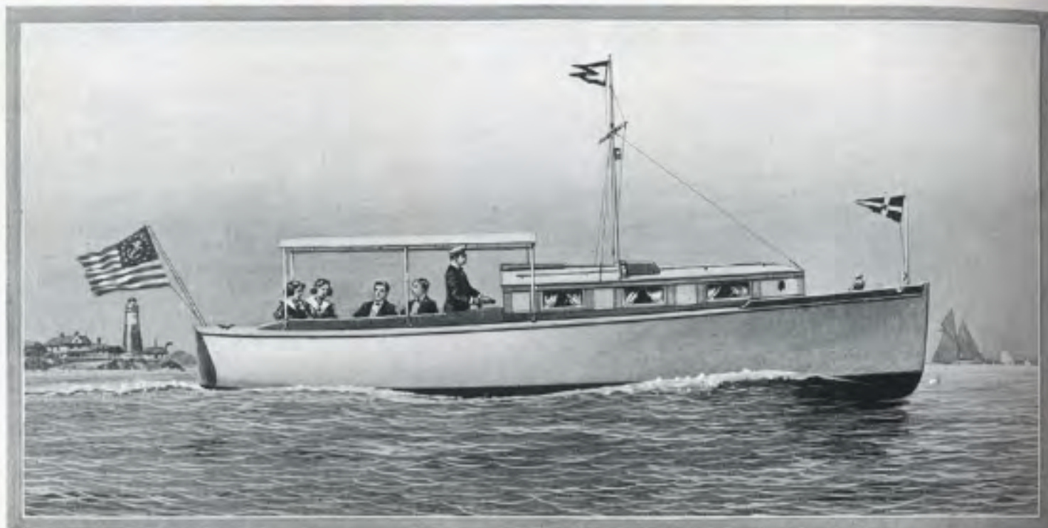
33-foot CRUISETTE, 36-40 Horse Power ELCO Engine, Speed 12 miles
