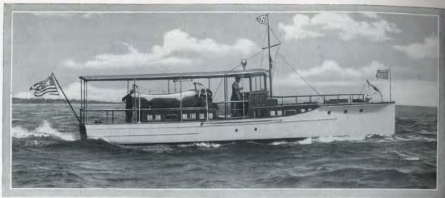
50-foot ELCO CRUISER, 75 Horse Power Engine. Speed 13 miles
