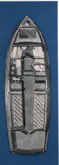
Forward cockpit formed by sunken deck. Easy and safe access from cabin through hatch. Stowage under for anchor gear.
