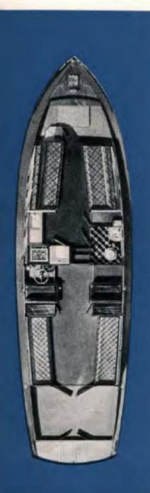
Forward cockpit formed by sunken deck. Easy and safe access from cabin. Shelves and anchor stowage under.
