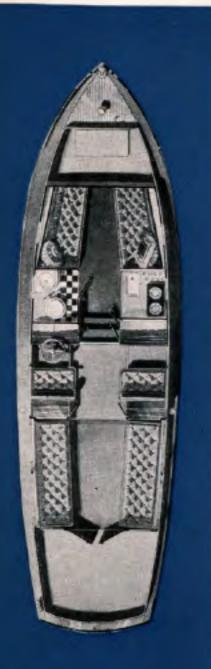
Forward cockpit formed by sunken deck. Easy and safe access from cabin. Stowage below for anchor gear.
