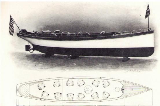
**36-FOOT ELECTRIC LAUNCH:** New Design with Floor Space for Chairs Extended to the Stern. Very popular for fair weather service, and can be fitted with long fly awning. Standard construction similar to preceding boat. Finished in mahogany. Standard No. 54 Power Equipment. Price: Open launch, as illustrated, without deck fittings and furnishings, F. O. B. cars, our works **\$2375 00**
