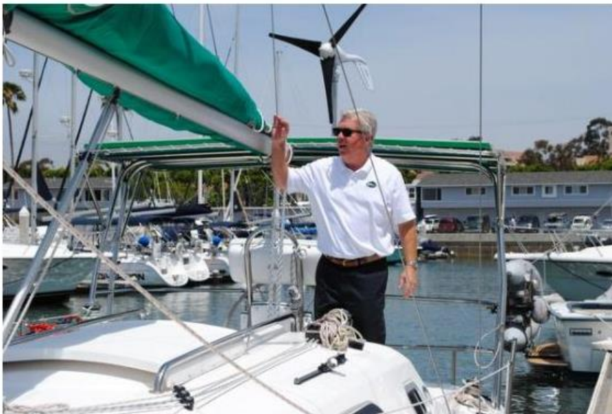
Kevin Kearns of Elco Motors explains how the wind turbine and solar panels aboard a Hunter sailboat charge the boat's 20-horsepower electric motor, creating a zero-emissions propulsion system.
